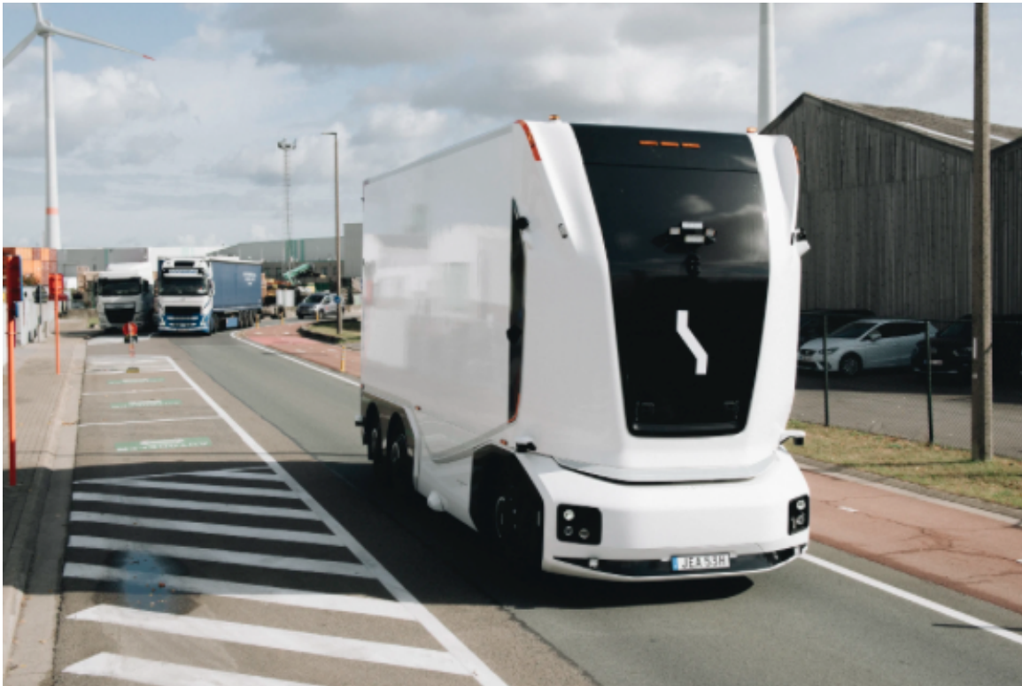
Abbildung 3 Einride autonomer Truck (Quelle: https://www.einride.tech/press/einride-operates-first-ever-fully-autonomous-heavy-duty-truck-on-a-public-road-in-belgium-at-the-port-of-antwerp-bruges )
